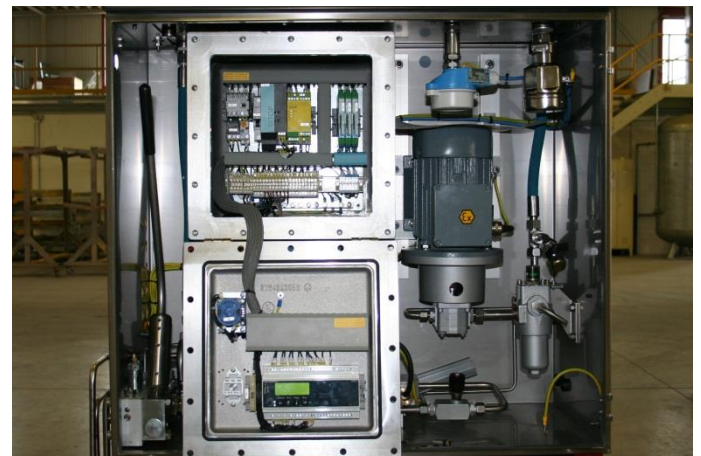
An IHP24-A with power unit control mounted on a self-contained system
