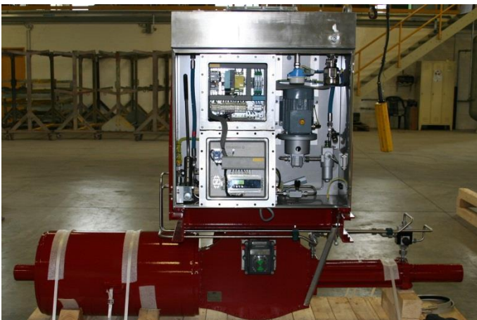
An IHP24-A with power unit control mounted on a self-contained system
